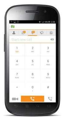
The *Dial pad* tab displays a dial pad and a text field used to enter numbers. The dial pad is one of the options used to make audio or video calls. There are three buttons below the dial pad: Call, Video call, and Dial pad menu that are configurable by the service provider. The top text field also has a delete button that, when pressed, deletes one character at a time.
